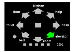
Fig. 2. P300 arrow paradigm. Each symbol is flashed during 100 ms and the time between flashes is 200 ms. Each arrow can be associated to a high level command.
