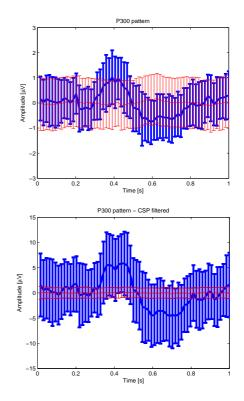
Fig. 4. Top: best channel mean and standard deviation over the set of target trial (blue) and nontarget trials (red); down: average and standard deviation of CSP filtered data from CPz, Pz, P3 and P4 channels.
