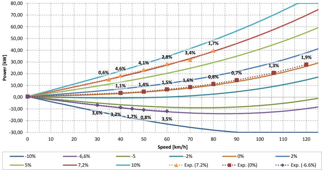
Figure 9: Power required to maintain a constant speed for several degrees of inclination and experimental runs (Exp.) on an average slope of 0%, 7.2% and -6.6%. The values near the experimental points correspond to the error, in percentage, between the mathematical model (Equation 10) and real data.
