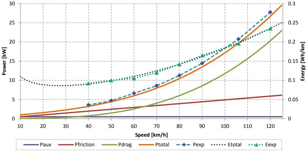
Figure 11: Details of the total power ( $P_{total}$ ) required to overcome each force acting on the vehicle ( $P_{aux}$ ,  $P_{friction}$  and  $P_{drag}$ ), in kW, and specific energy consumption ( $E_{total}$ ) for a flat surface, in kW/km. Power (Pexp) and specific energy consumption (Eexp) from experimental runs are also presented.
