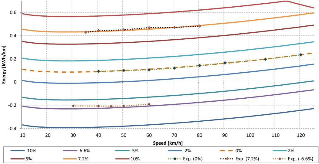
Figure 10: Energy consumption per unit of distance required to maintain a constant speed for several degrees of inclination and experimental runs (Exp.) for 0%, 7.2% and -6.6%.
