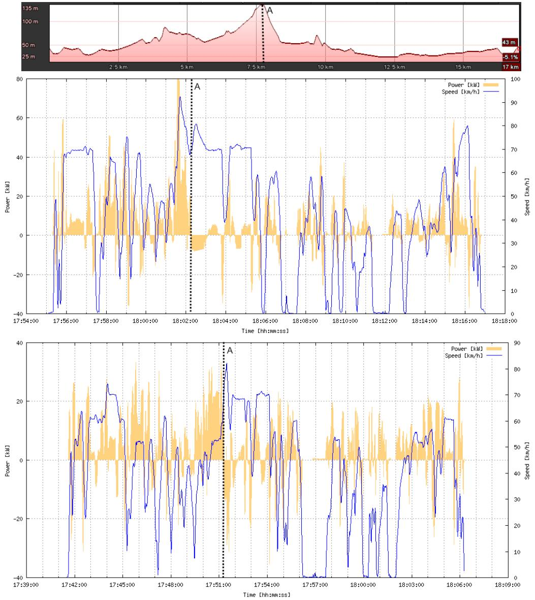
Figure 12: Power and speed for a mixed driving cycle in urban and extra-urban environment for a 16 km trip with the elevation profile represented on top, in a Normal (middle graph) and ECO (bottom) driving styles. The power consumption with negative values, in parts of the driving cycle, is associated with regenerative braking.
