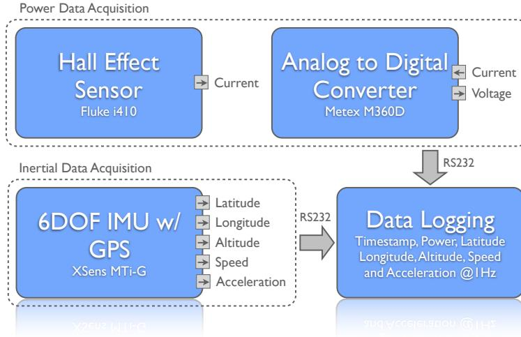
Figure 8: Data acquisition system installed on a Nissan Leaf.
