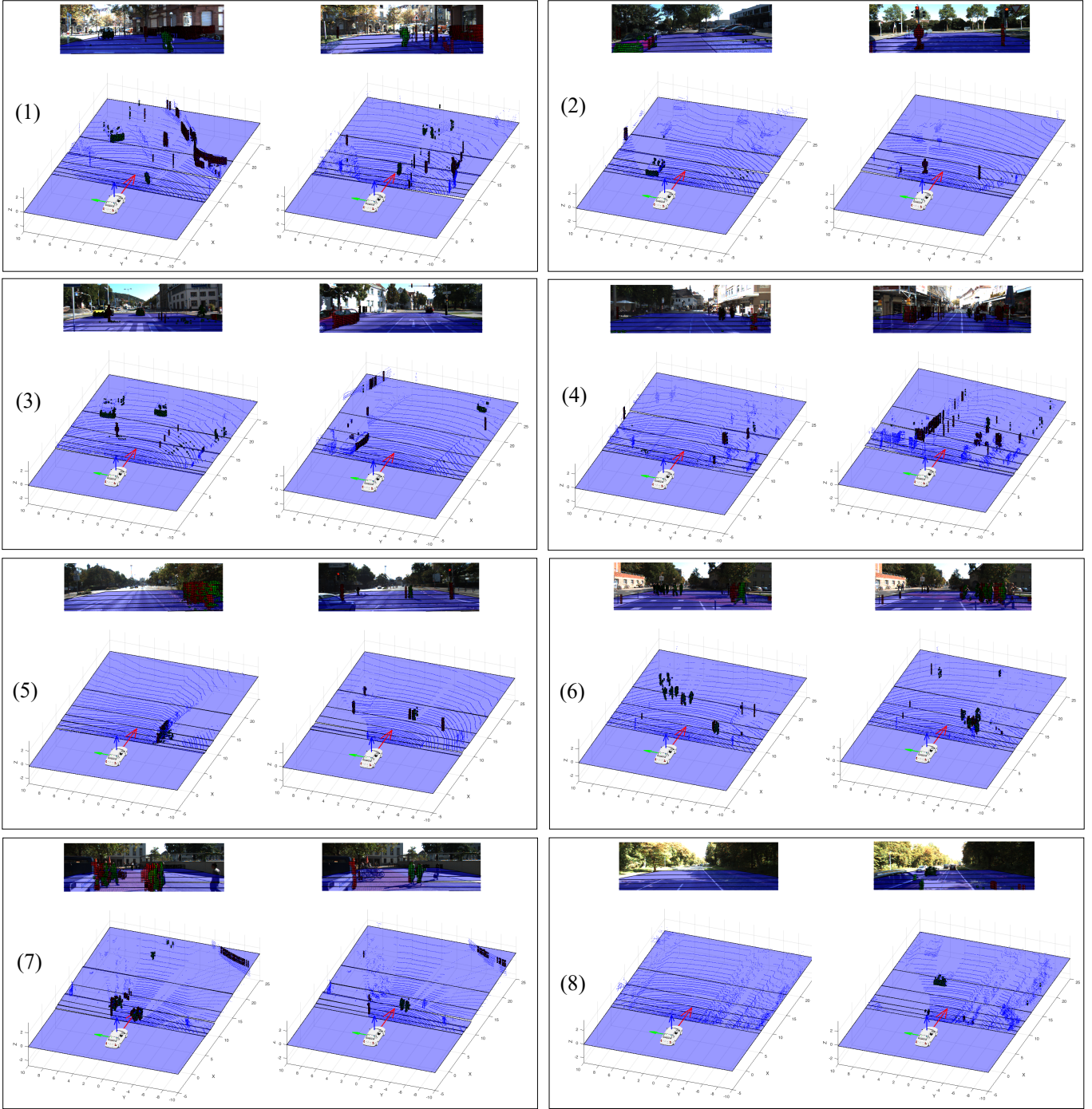
Figure 11: Sample screenshots of obstacle detection results obtained for sequences 1 to 8 as listed in Table 2 and its corresponding representation in 3D. Piecewise ground planes are shown in blue. Stationary and moving voxels are shown in red and green respectively.
