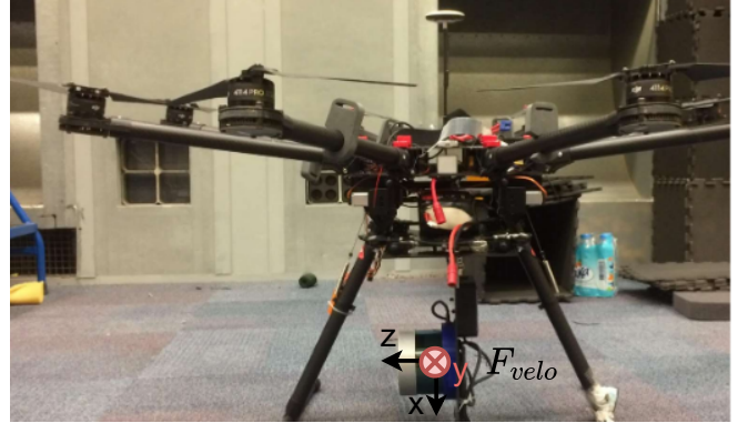
Fig. 1. The octocopter drone (DJI S1000) with the onboard LiDAR (Velodyne VLP-16) used to collect point cloud data for human detection. The sensor coordinate reference system ( F_{velo} ) are designated by the xyz axes.
