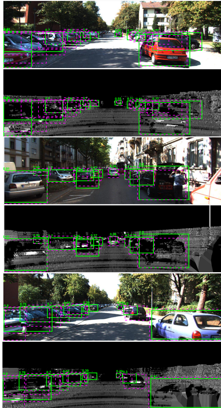
Fig. 5. Example screenshots of RefCN results. Detection results are shown, as green BBs in the color-images (top) and DRMs (bottom) compared to the ground-truth (dashed-magenta). Notice that the depicted color-images are shown only for visualization purpose.
