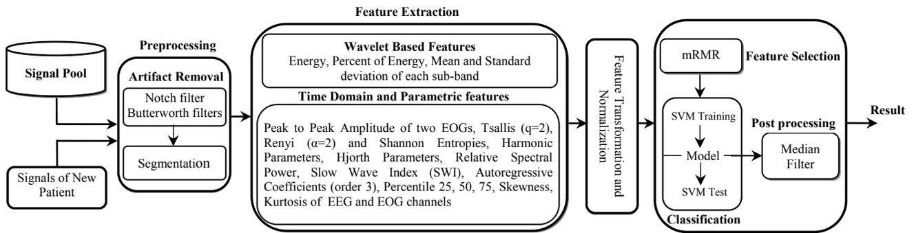
Fig.1 System Architecture
