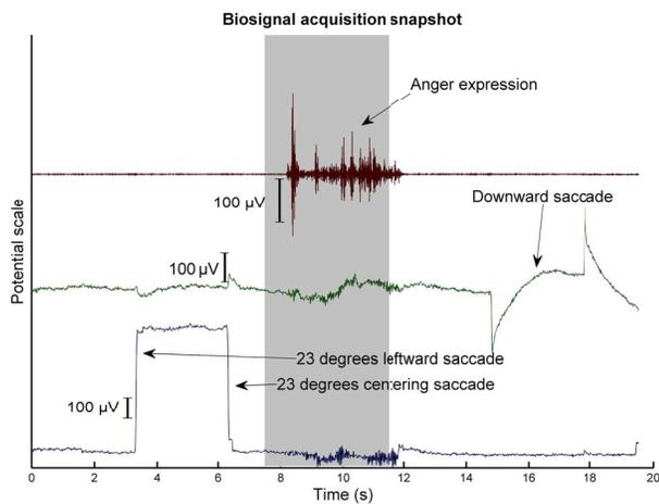
Fig. 2. A superimposed trace of simultaneous horizontal EOG (bottom trace), vertical EOG (middle trace) and *Corrugator supercilii* EMG (top trace) during three different, sequential actions: a horizontal saccade, followed by a facial expression, followed by a vertical downward saccade. Note how the EMG signal originates crosstalk on both EOG sources when an expression is made (shaded area).
