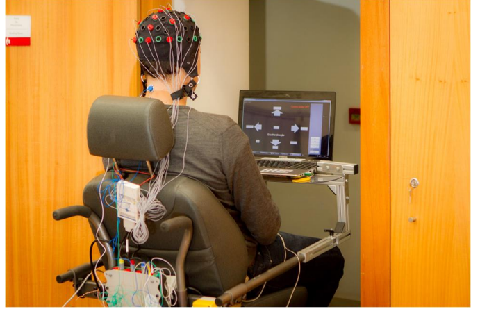
Fig. 1. Snapshot taken during an experiment with an able-bodied participant steering RobChair with the self-paced P300-based BCI.
