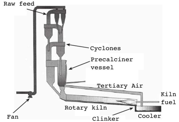
**Figure 1:** A diagram of a cement rotary kiln plant, adopted from [19].
