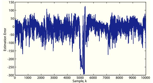
**Figure 6:** Estimation error in degree Celsius between the measured burning zone temperature and the unscaled neural network output in the cement kiln process.
