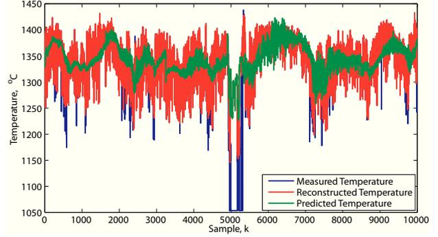
**Figure 5:** Measured burning zone temperature, reconstructed burning zone temperature using the proposed methodology and the unscaled neural network output in the cement kiln process.
