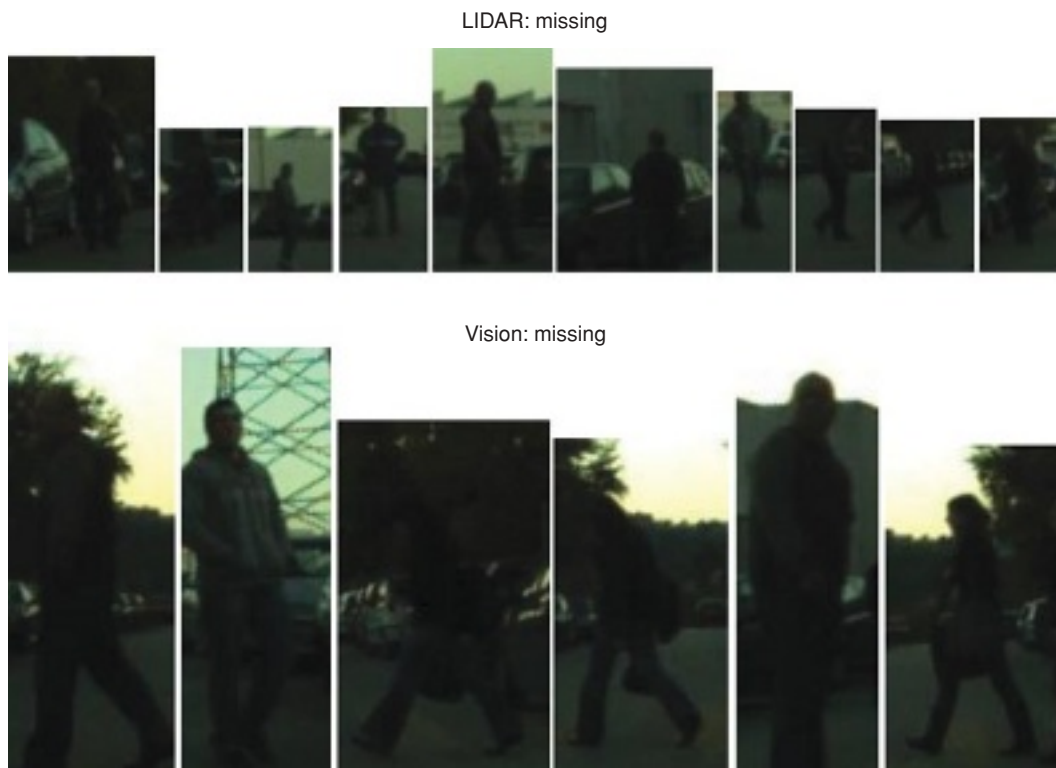
Figure 6. Some examples of miss detections using single classifiers: the LIDAR–naive and vision–LDA.
