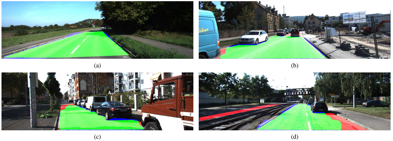
Fig. 5. In (a) we have an example of a road without obstacles, while in (b) and (c) there are vehicles on the road. Finally, in (d) there is a difficult case where the road in the left part is considered ground-truth, which we had a complete missing (red color).
