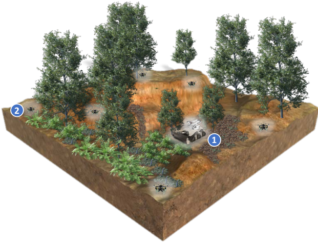
Fig. 2. Illustrative deployment of the SEMFIRE solution. 1) the powerful multi-purpose Ranger can autonomously mulch down the thickest brushes as well as cutting down small trees to reduce the risk of wildfires; 2) the area is explored (finding new regions of interest with forest debris) and patrolled (checking the state of these regions of interest) by Scouts, having the additional task of estimating the pose of each other and the Ranger and supervising the area for external elements (e.g. living beings).
