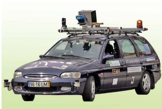
Figure 2. An instrumented car developed by the University of Aveiro.
