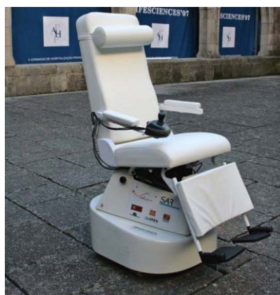
Figure 5. Autonomous mobile chair, which is a commercial product developed by a spin-off robotic company from the University of Minho.
