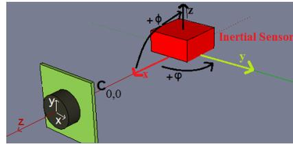
**Fig. 3.** Inertial and camera  $C_{0,0}$  referential
