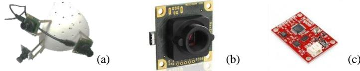
**Fig. 4.** Hardware used on the trials, (a) 3D printed version of part the Sphere (b) UI 1226LE-M camera from IDS-Imaging (c) 6DOF Inertial Measurement Unit.
