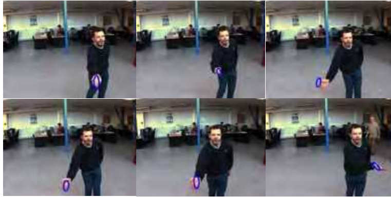
Figure 11. 3D tracking of a hand in heavy clutter. The blue (resp. red) ellipses depict the particles (resp. the MMSE estimate). Automatic re-initialization after target loss
