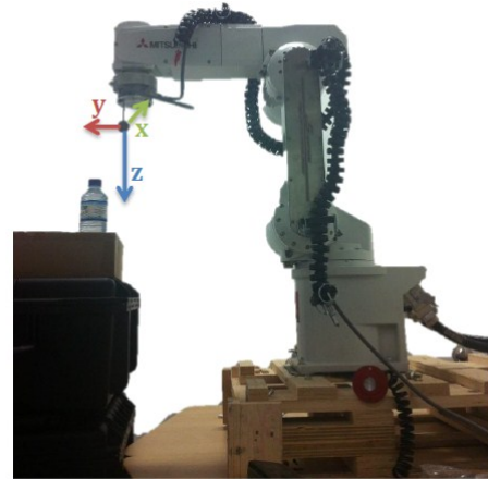
Figure 2: Experimental setup (Mitsubishi Arm + F/T sensor + sphere + object)
