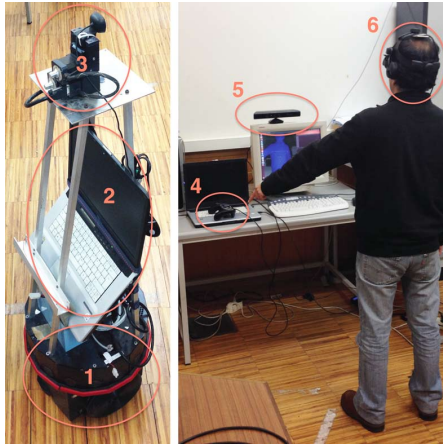
Fig. 4: Hilario Robot (left) and Remote Control Station (right): (1) Scout, (2) Laptop, (3) PTU Camera, (4) Joystick, (5) RGB-D Camera, (6) Head-Mounted Display
