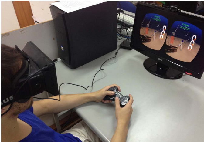
Fig. 5. The participant is running an experiment (setup 2). The HMD will use the splitted imaged display in the screen to generate the 3D image.
