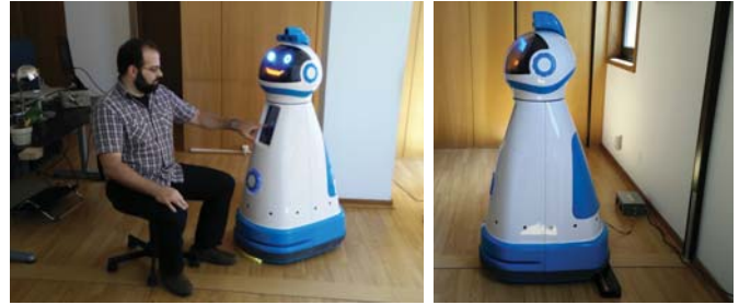
Figure 2: The service robot platform developed: a) Human-Robot Interaction; b) Docking Station.
