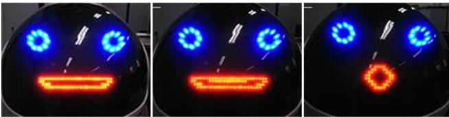
Figure 4 - GrowMeUp robot mouth shapes for the word "Hello".
