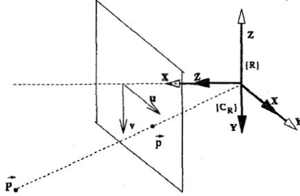
Figure 5: The camera referential and picture coordinates.
