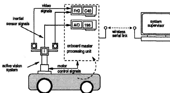
Figure 3: System Architecture. The inertial system processing board uses the Master processing unit as host computer.
