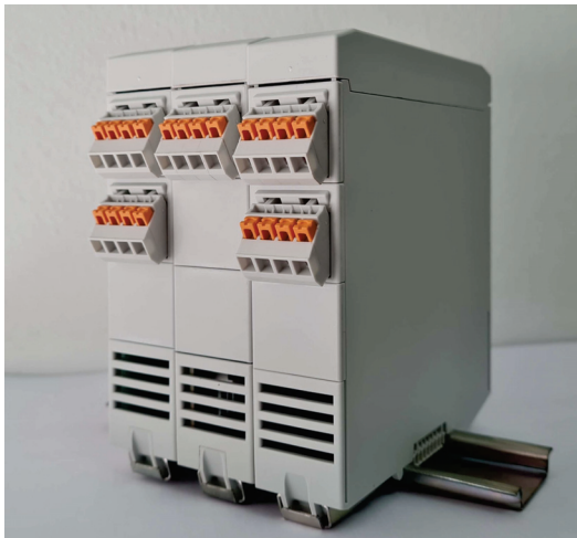
Figure 12. Industrial Control System developed with expansion modules coupled.
