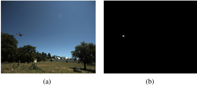
Fig. 5: (a) Detected drone, marked with a red dot (b) The corresponding binary mask
