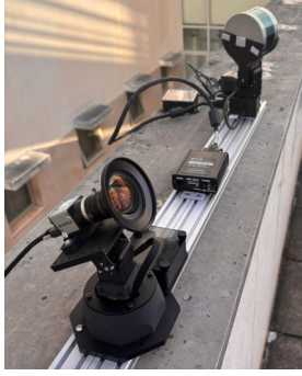
Fig. 4: Drone detection setup with the Velodyne VLP16 on a PTU 46-17.5 and the camera on a PhantomX XL430
